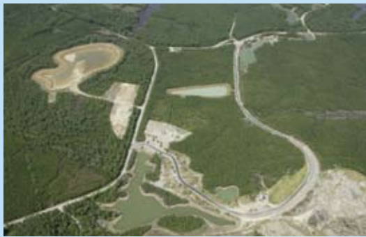
The three infiltration basins at River Dunes, shown above, have a combined capacity of 0.321 mgd. The treatment facility can accommodate 0.5 mgd. The Bay River Metropolitan Sewerage District, which supplies wastewater treatment to the area, is planning additional basins adjacent to the new reclaimed water pipeline that will connect the wastewater treatment facility to the infiltration basins at River Dunes. This system should be completed by the end of 2008.
